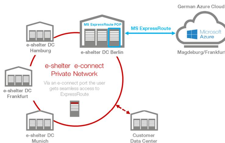
Figure: End-to-end Microsoft German Azure Cloud at e-shelter data centers (DC)
